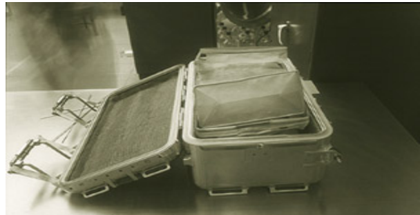
Fig. 1. Apollo Lunar Sample Return Container (Moon Box) open showing plastic bags to segregate lunar material.
