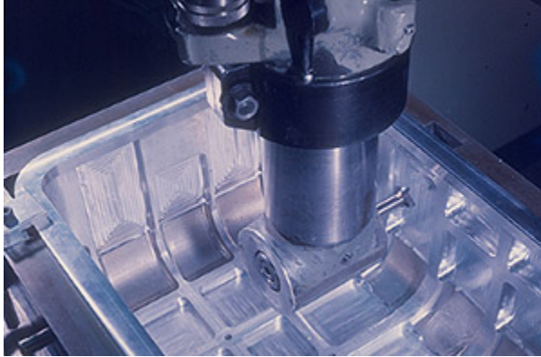
Fig. 2. Machining the inside dimension and creating the rib construction for added strength on a milling machine at Y-12.
