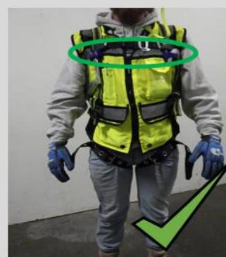
Retention devices installed at chest level
