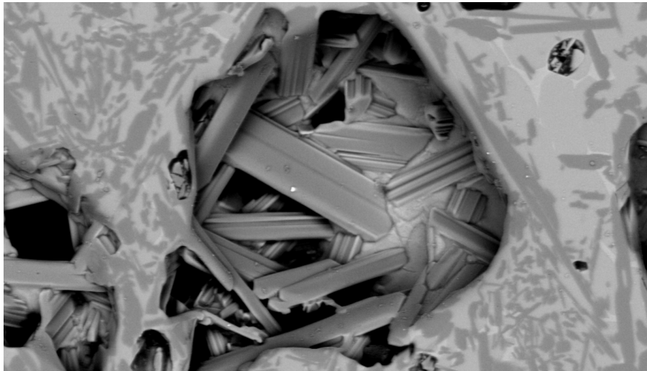
▲ Microscopic view of needles in TiBor Skin composite structure.
