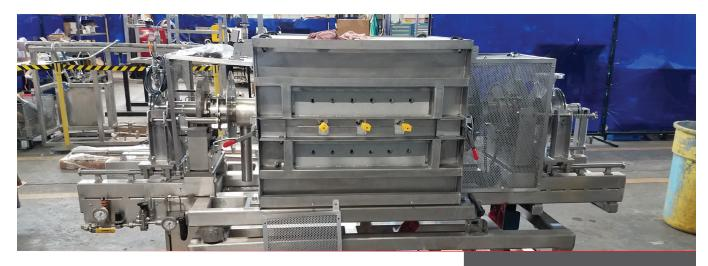
The Calciner Project (CALP) is key to phasing out mission dependency on Building 9212. It provides Y-12 with a calcination process capable of converting low-equity uranium solutions into a solid form for safe storage.
